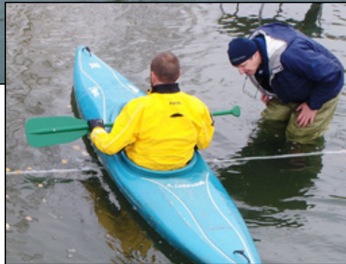
Left: An old-school kayak passes over the Mirror Lake boat-draft measuring bar (4-inch draft with 160 lbs.).
