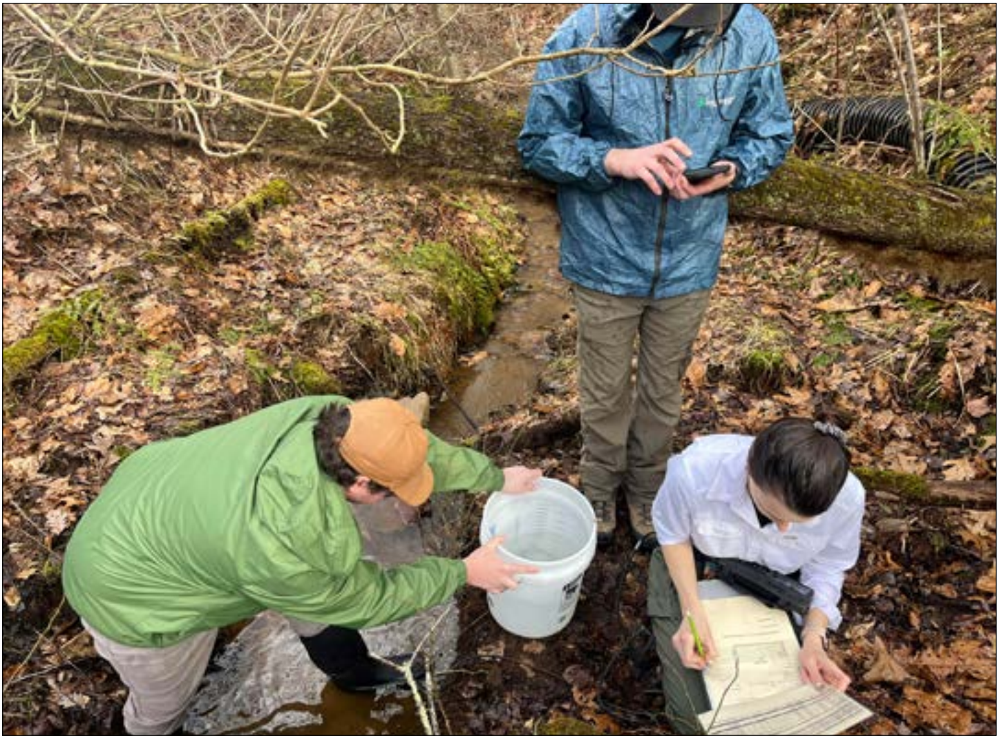
Learning with Local Groups: Measuring flow using the bucket method at one of Friends of Decker’s Creek’s rare earth element sampling sites. Photo: Abby Walters-Gonzalez
