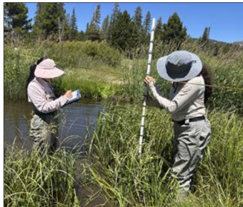
Measuring the Flow: Collecting cross-sectional stream channel data in Van Norden Meadow. Photo: South Yuba River Citizens League
