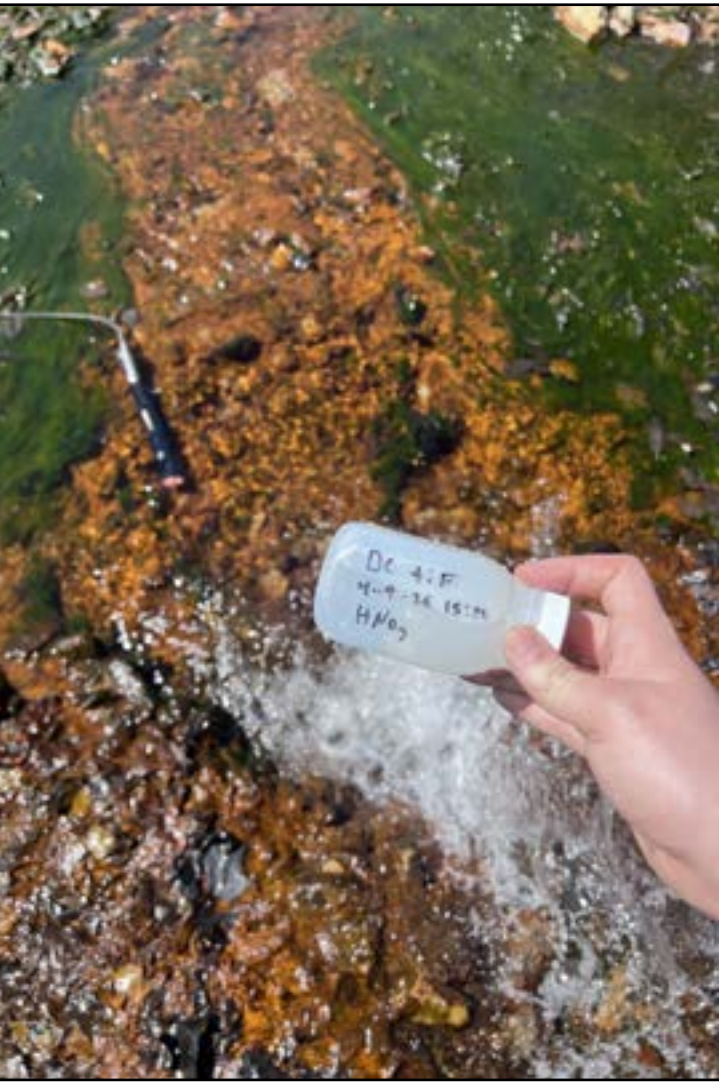
Water Sample Collected at Polluted Site: Water sample collected utilizing the YSI probe in order to collect streamflow statistics like pH, specific conductivity, and temperature (note: coloration and plant growth).
