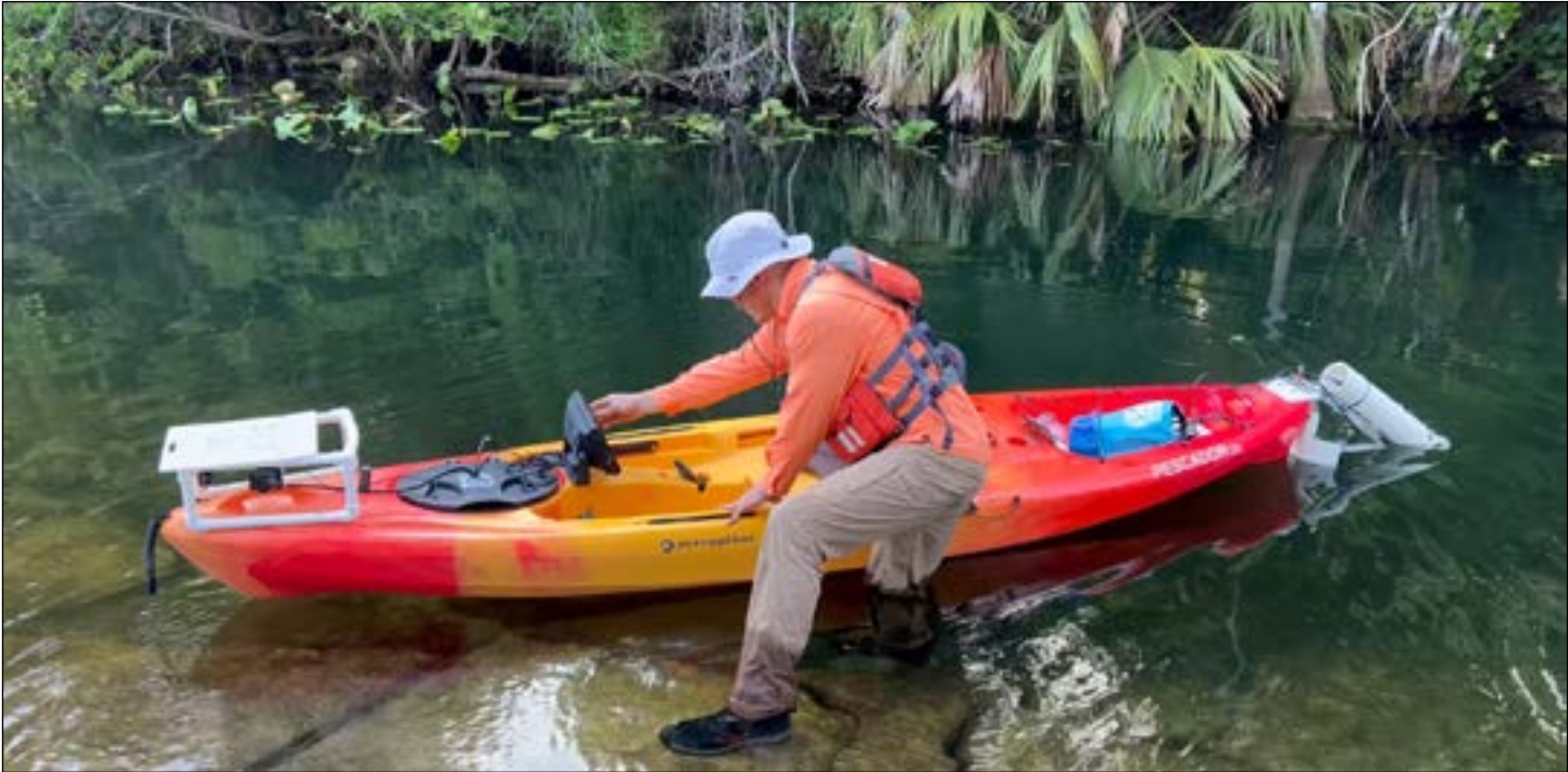
Below and opposite: Mapping Watersheds With High-Tech Boats. The High Definition Stream Survey (HDSS) utilizes multiple survey platforms to efficiently document stream corridors across a wide range of conditions. Wadeable streams are surveyed using a backpack system equipped with georeferenced video and water quality monitoring equipment, while kayaks and inflatable rafts support data collection in deeper waters. Together, these platforms allow HDSS to collect continuous georeferenced video, bathymetry, side scan sonar, and water quality data from headwater streams to large river systems, creating a consistent baseline dataset across the entire watershed. Photos: Brett Connell/Trutta Consulting
