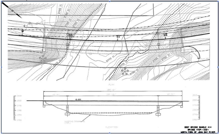
N Bridge - The superstructure would be supported on piers located above the ordinary high water elevation and end bents at each end of the bridge founded on rock.
